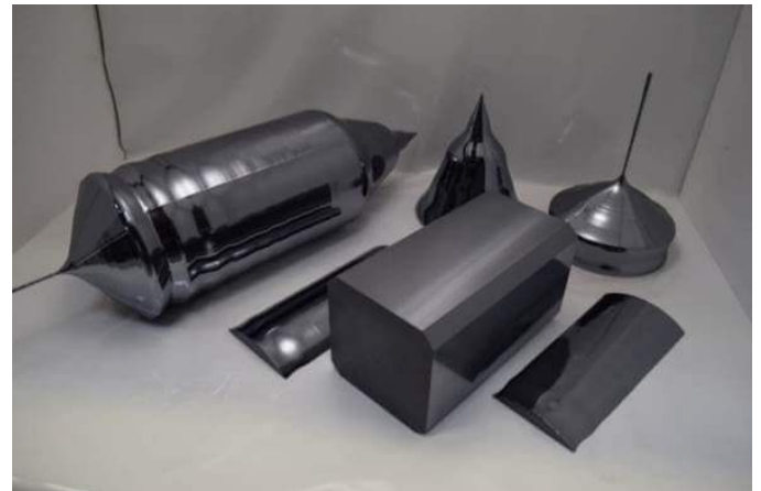
Czochralski process whole ingot (left), and brick and chords after sawing (right), crown and tail (upper right) ( SVM )
