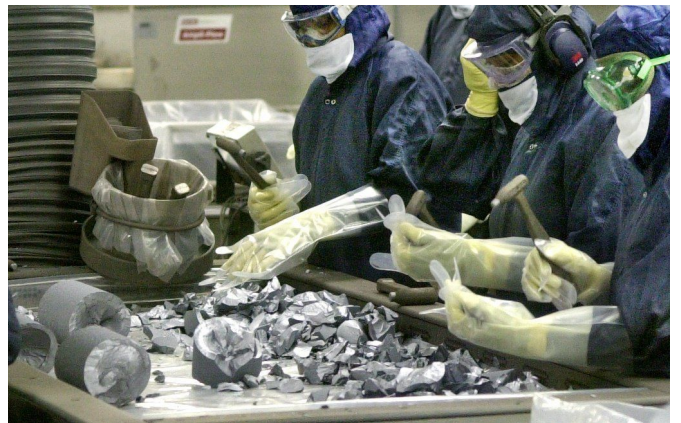
Polysilicon rods and sections being broken into chunks by hand in a clean room. (Hemlock)
