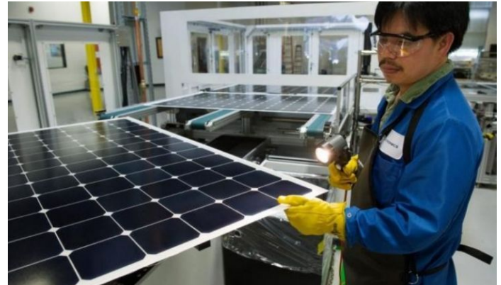
Solar module inspection on the assembly line. (Solar World)
