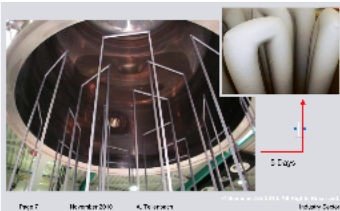
Left: When heated to around 1100°C the polysilicon “filaments” standing beneath the reactor cover can “catch” about 20% of the silicon atoms that pass through the reactor in gaseous form. Right: Polysilicon “rods” after 5 days of growth. (Siemens AG)
